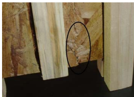
Fig. 8 OSB tore in shear near application line
