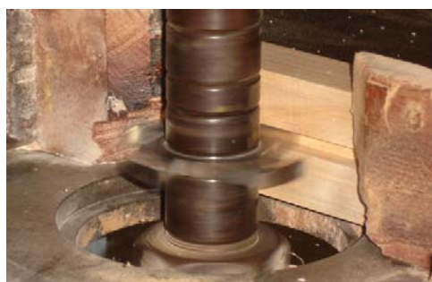
Fig. 4 Mortising machine producing the rectangular groove
