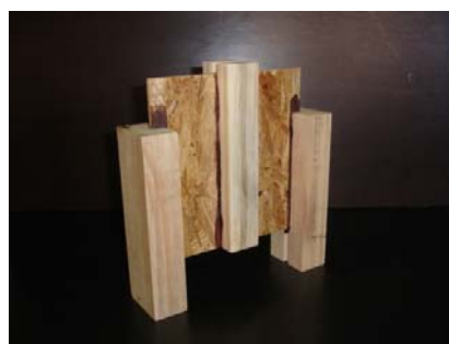
Fig. 6 Web-to-flange joint specimen with reinforcement
