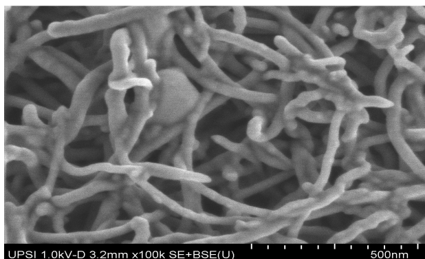
Fig. 8 FESEM images of MWCNTs-calix[8]arene with \text{Cd}^{2+}
