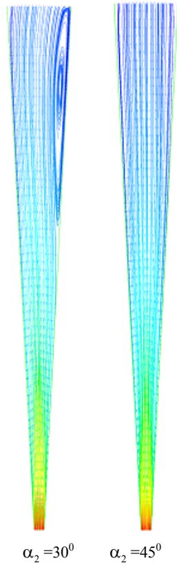
Fig. 9 Meridian configuration of the conical diffuser with \bar{b}_2 = 0,014 and \vartheta = 6^\circ . Meridian streamlines are presented at two inlet angles. \bar{D}_3 = 1,60, \lambda_{c2} = 0,64, Re_{D2} = 9,1E6
