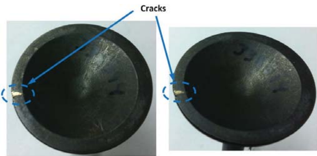
Fig. 2 Cracks at the "blade" area after coining
