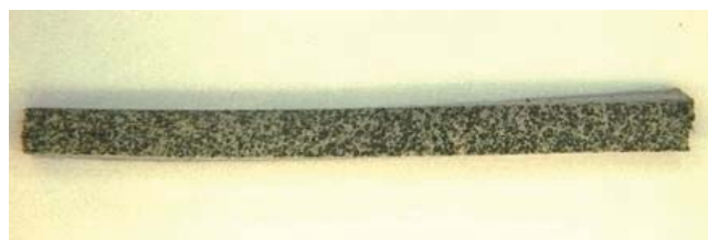
Fig. 3 A strip of the epoxy modified with rubber sample after 2 months exposure to deionized water at 80°C and complete drying
