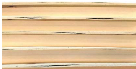
Fig. 12 Specimens prepared from polyester material immersed in water at 80°C for two months and after drying shows how delamination has happened along the edges
