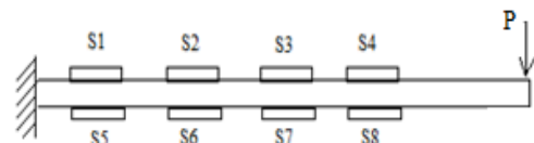
Fig. 2 Schematic showing numbering of strain gauges
