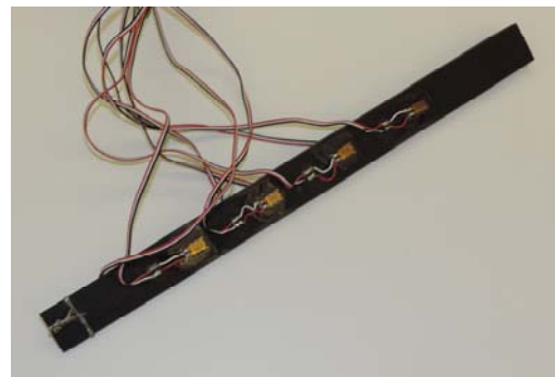
Fig. 3 Test specimen for measuring bending stresses
