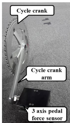
Fig. 1 Three-axis Pedal Force Measurement Sensor installed Device
