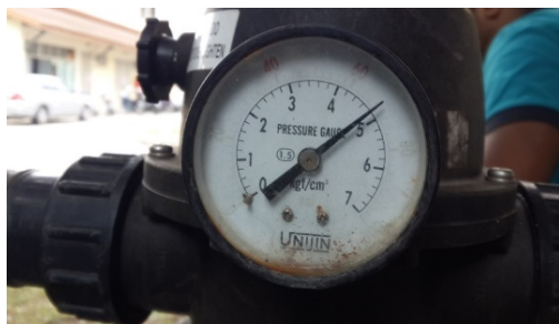
II. FIG. 3 WORKING PRESSURE READING ON THE PRESSURE GAGE EXPERIMENTAL WORK
