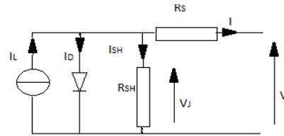
Fig. 3 Equivalent circuit of a solar cell
