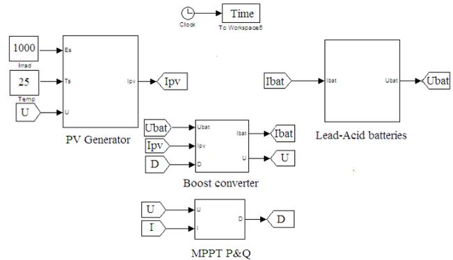
Fig. 8 PV system controlled by MPPT algorithm
