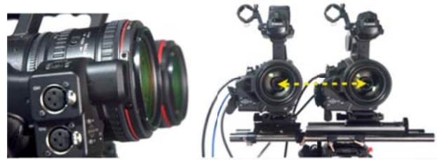
Fig. 13 Stereo camera: interaxial separation
