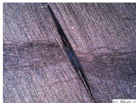
Fig. 1 Fish-Eye in a NCF in matrix made of carbon fibre; polyester binding yarn
