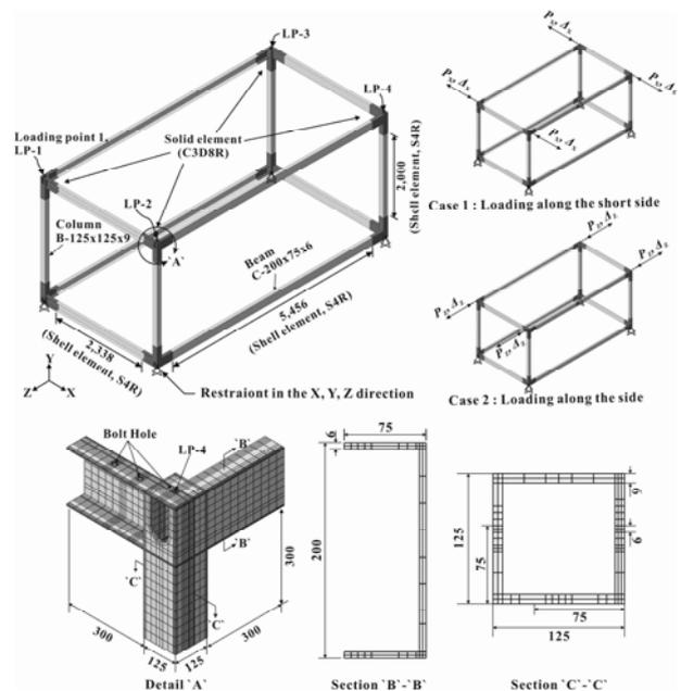
Fig. 1 Detailed boundary conditions and geometry of a FEM model
