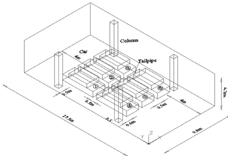
Fig. 2 Model geometry in the study: Number 1-6 in the figure represent car number in the model
