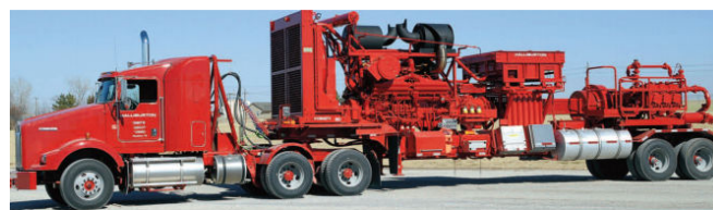
Fig. 1 Typical fracturing pump trailer
