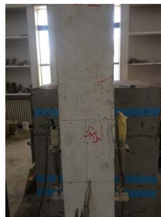
Fig. 3 Failure of control specimen
