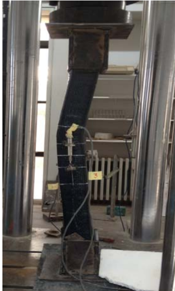
Fig. 4 Failure of CFRP wrapped specimen (NE)
