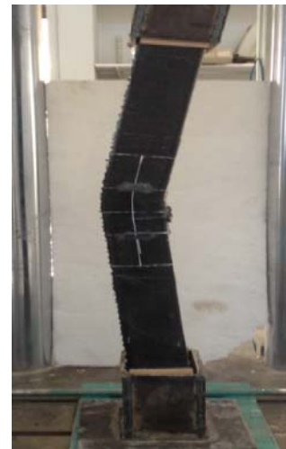
Fig. 6 Failure of CNTE specimen
