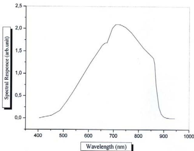
Fig. 1 Spectral response of (n-AlGaAs/p-GaAs) solar cell [4]
