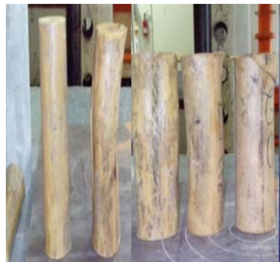
Fig. 4 Mixed modes of failure observed in samples
