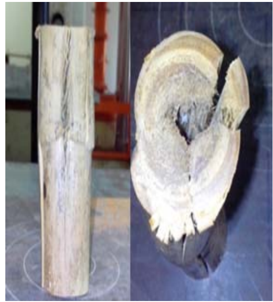
Fig. 3 Cracking and splitting mode of failure
