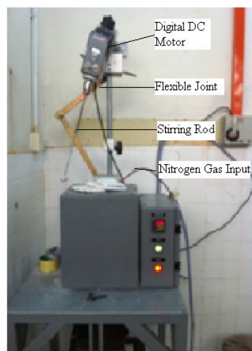
Fig. 1 Fabrication of metal matrix composite was using the stir casting technique. The stir casting equipment was built in-house
