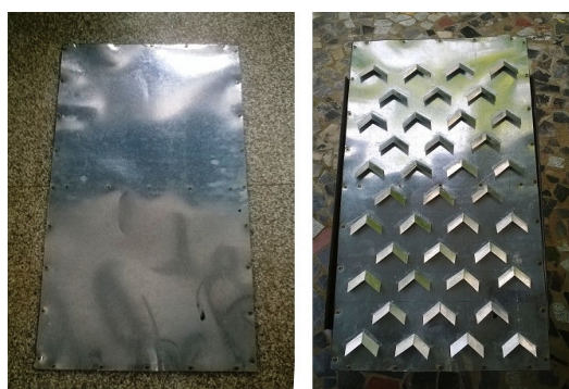
Fig. 3 Smooth and roughened absorber plate
