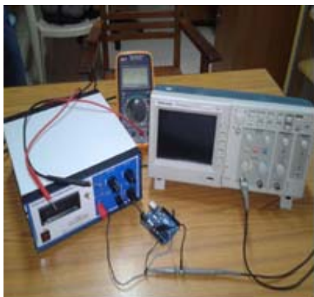
Fig. 9 (b) Testing set up of Arduino Mega 2560
