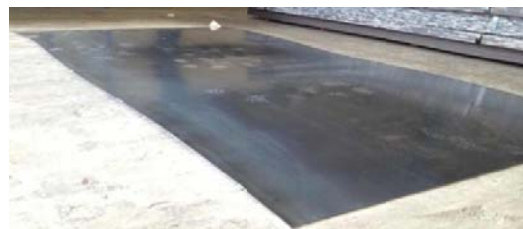
Fig. 3 Sample of edge waviness defect
