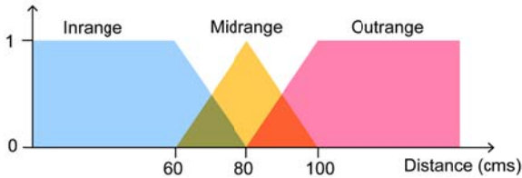
Fig. 3 Input membership functions for laser reading sensors
