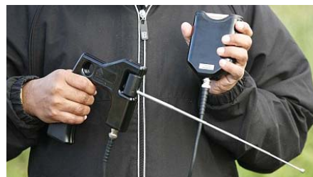
Fig. 1 The 'bomb detection' device is supposedly powered by static electricity [3]
