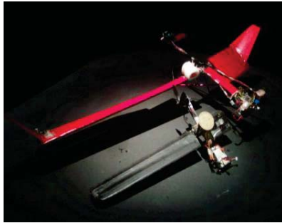
Fig. 1 Monocopter systems constructed
