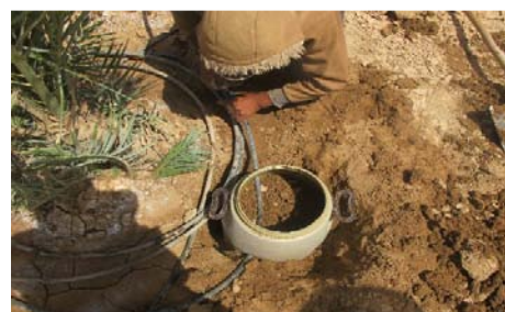
Fig. 4 Bin Used to Measure the Distribution Uniformity and Evaporation Water Losses
