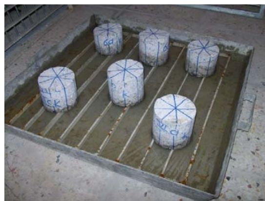
Fig. 4 Capillary water absorption experiment
