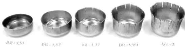
Fig. 1 Delayed cracking after deep drawing of austenitic stainless steel with different drawing ratio [1]
