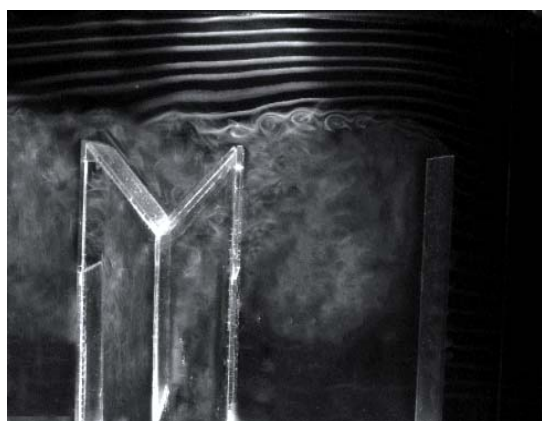
Fig. 12 Visualized flow pattern around and inside the two-sided wind-catcher with upstream structure ( h=H & X=0.75H )
