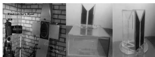
Fig. 8 Experimental setup and wind-catcher model
