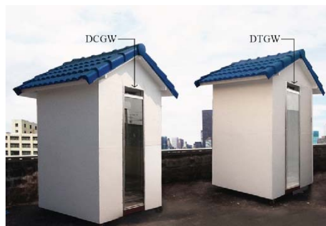
Fig. 1 The double glass wall models in the experiment (DCGW and DTGW)
