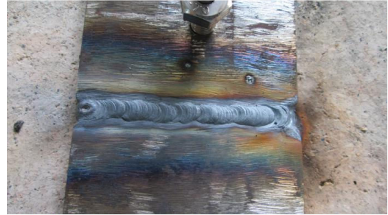
Fig. 5 A close view of weld bead and heat affected zone
