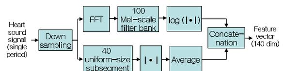
Fig. 4 Feature extraction for ELM-based classifier.
