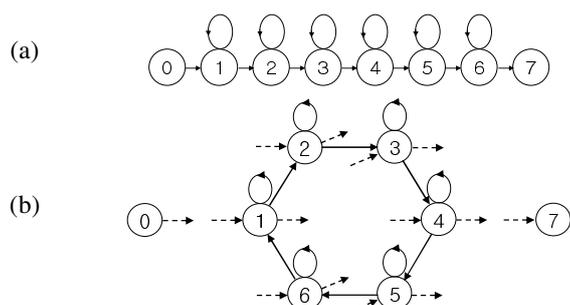
Fig. 6 The structure of (a) the left-to-right and (b) the circular HMMs.
