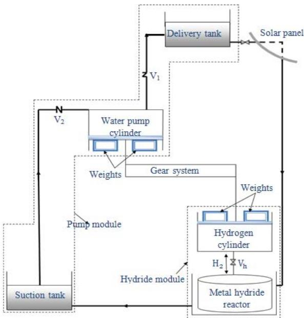
Fig. 1 Schematic of metal hydride water pumping system
