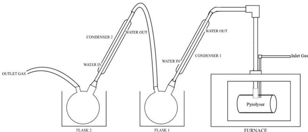
Fig. 1 Experimental set up for slow pyrolysis process
