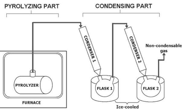
Fig. 1 Schematic diagram of slow pyrolysis set-up
